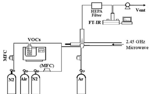
Fig. 17. Schematic layout of the benzene-removal experimental setup.
