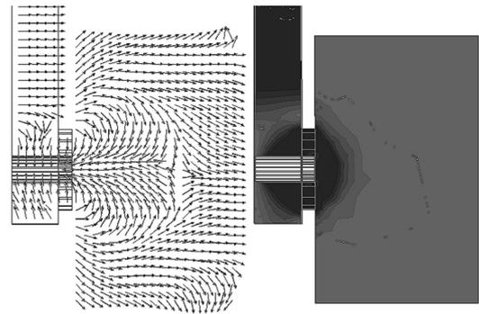
Fig. 7. (Left) Distribution of the electric field lines and (right) the contour plot of the electric field in the waveguide and the radiation region
