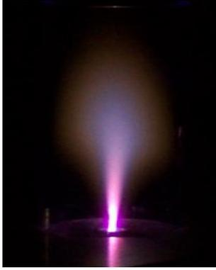
Fig. 13. Torch-flame and background plasma inside the quartz tube.
