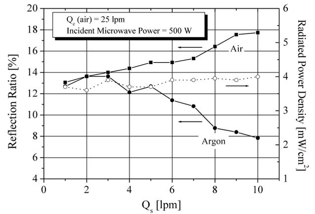
Fig. 10. The effect of the side gas flow rate on the power reflection and the radiated power density. The incident microwave power is 500 W, and the air gas flow rate of the center nozzle is 25 lpm. The radiated power density is measured for the argon gas.
