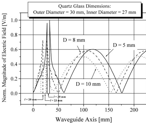
Fig. 6. Normalized magnitudes of the electric field on the waveguide axis, the waveguide-center line in the parallel direction to the propagating wave, for various nozzle diameters.
