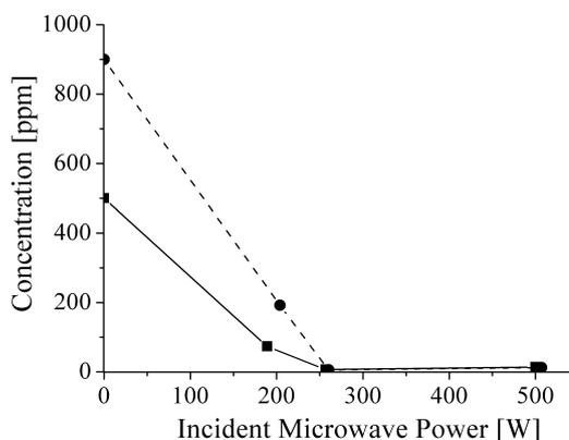
Fig. 19. Removal characteristics of high levels of benzene as a function of the incident microwave power.
