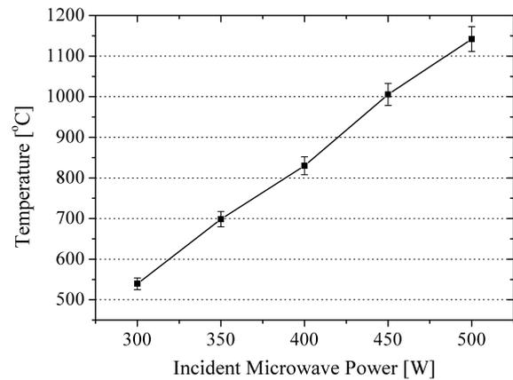
Fig. 11. Temperature at 10 cm from the nozzle, as measured using a B-type thermocouple, as a function of the incident microwave power. The argon gas flow rate is fixed at 4 lpm.
