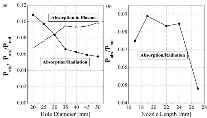
Fig. 5. (a) Absorbed power in the plasma and its ratio to the radiated power as functions of the hole diameter, and (b) the ratio of the absorbed power to the radiated power as a function of the nozzle length. In (a), the scale of the ratio of the absorbed power to the radiated power is adjusted to be compared with the power absorbed in the plasma.
