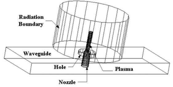
Fig. 4. HFSS model for calculating the absorbed power and the radiated power in the torch region.
