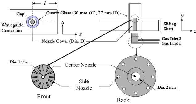
Fig. 3. Schematic drawing of the coaxial-field structure of the torch system.
