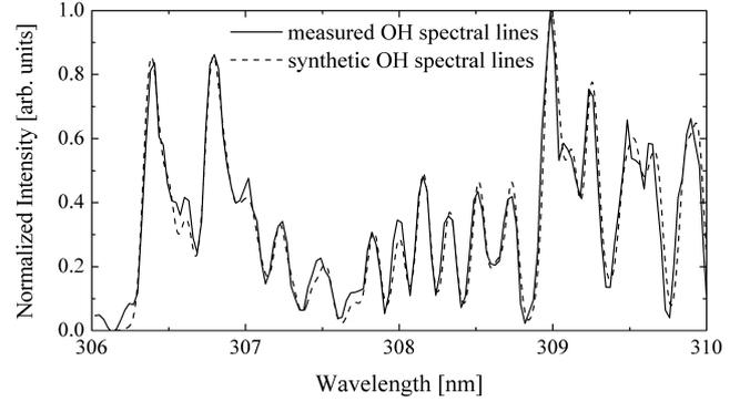
Fig. 14. The measured OH spectrum (solid line) and the synthetic OH spectrum for the rotational temperature of 4500 K (dashed line).
