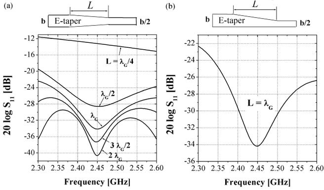
Fig. 2. Reflection of two kinds of tapers as functions of the frequency for various taper lengths.
