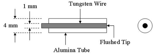
Fig. 15. Geometry of the single Langmuir probe.
