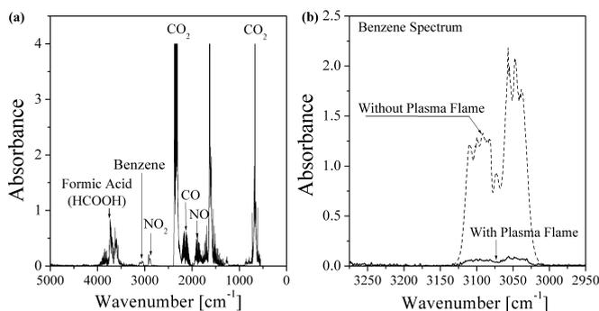
Fig. 18. (a) Measured FT-IR molecular spectra of a mixed gas after passing through the plasma flame. Here, the microwave power is 200 W. (b) Magnified view of the benzene peaks with and without a plasma flame. Benzene is removed significantly by the plasma flame. Here, the microwave power is 500 W.
