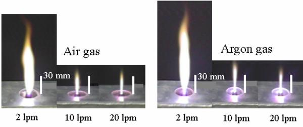
Fig. 12. Air and argon torches are compared for various flow rates for an incident microwave power of 500 W. Rulers of 30 mm are shown at the right side of each torch figure.
