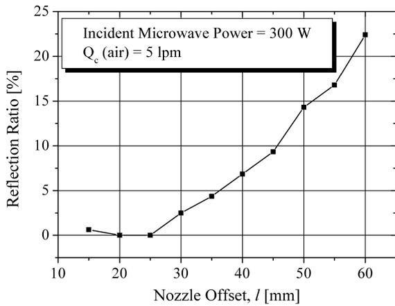
Fig. 8. Reflection ratio as a function of the shorting-plate position. The incident microwave power is 300 W, and the air gas flow rate is 5 lpm.
