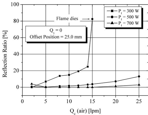
Fig. 9. Dependence of microwave power reflection on the air flow rate of the center nozzle without side gas feeding.
