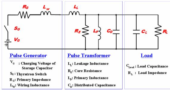
Fig. 1. Equivalent circuit of pulse transformer.
