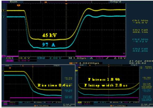
Fig. 6. Load voltage and current waveform with 472  $\Omega$  resistor (ch 2 (1000X), ch 2 (10X)).
