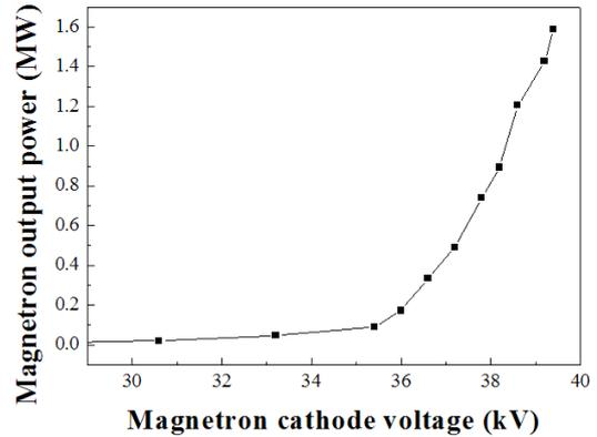
Fig. 8. 5-GHz RF output power *vs.* magnetron cathode voltage.
