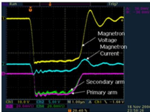
Fig. 7. Waveforms of magnetron cathode voltage and current and RF detector output voltage in two splitting arms.
