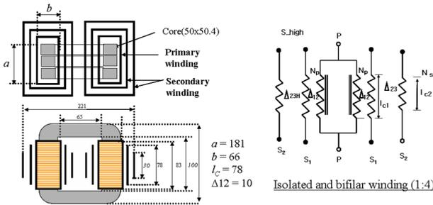
Fig. 2. Coil geometry and winding configuration.
