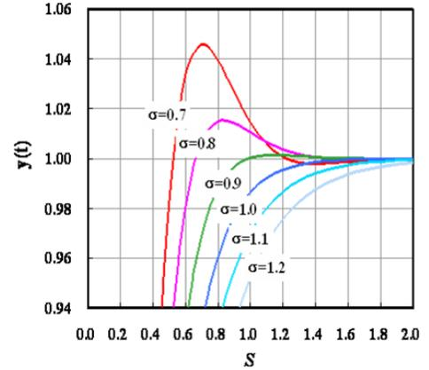
Fig. 3. Normalized rising-pulse waveform for various values of the damping factor.
