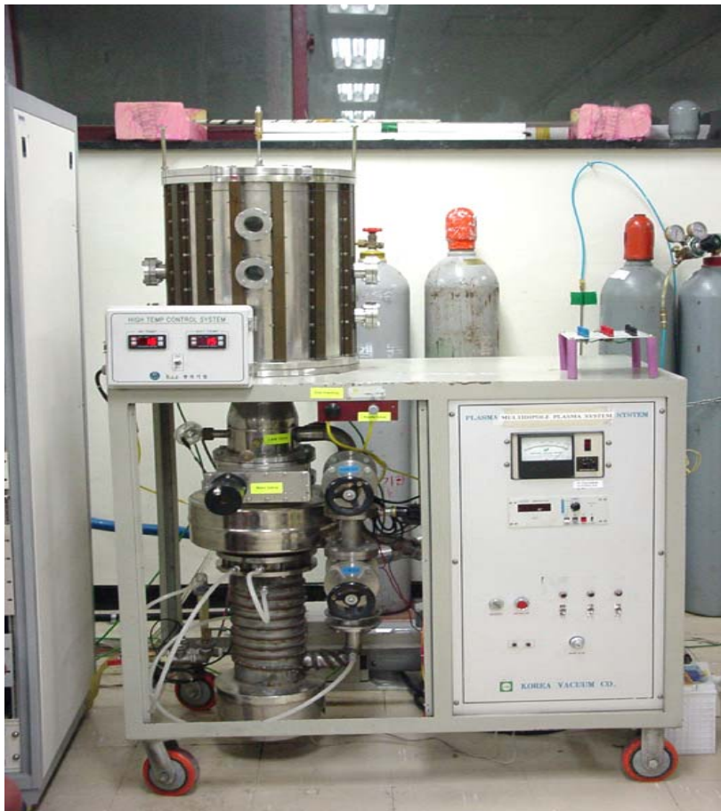
Multi-dipole Chamber System
