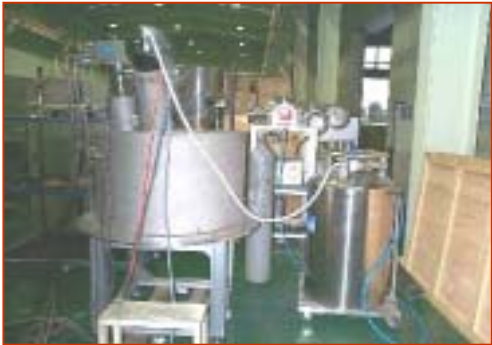
Filling of LN2 Compressor & Cryo-cooler on Pre-cooling with LN2
